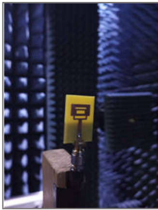
Fig.5. Measurement of Fabricated Antenna in Anechoic Chamber
